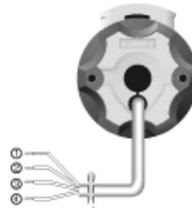
2. **110-volt AC motors cannot be wired in parallel** and multiple motors cannot be wired to a single pole switch. Directional leads must be isolated from one another. Failure to isolate the directional leads will burn out the motor.
